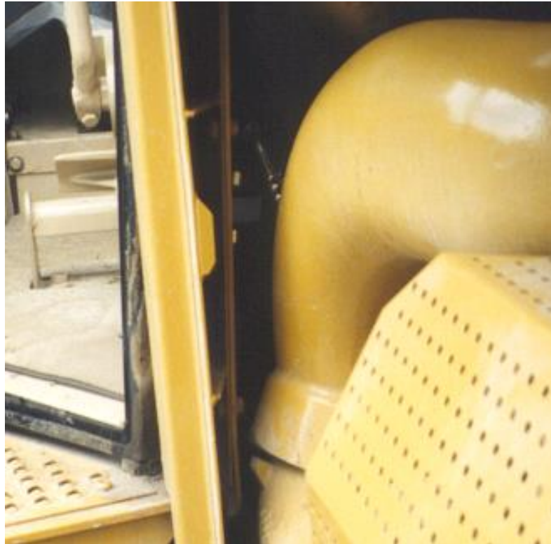
Drier location on side of rear engine compartment.
