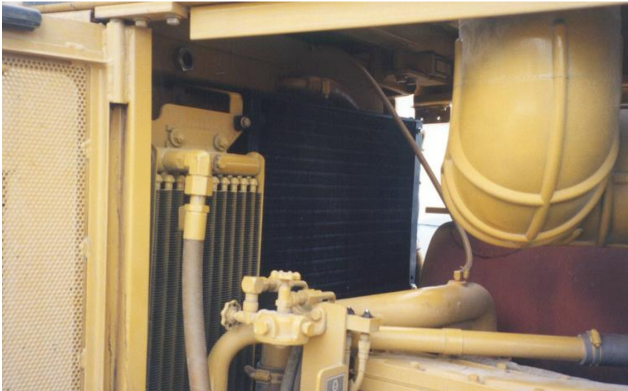
Left side of condenser assembly.
