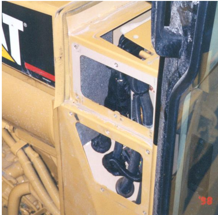
Evaporator assembly showing hoses.
